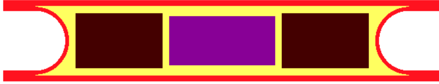
Figure 3.3: Cross section of the Theragenics Model 200 ( ^{103}\text{Pd} ) seed. Drawing is to scale and a detailed description is given in the text.
